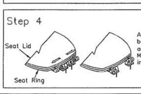
Attach the hinge mechanism to the seat, both the hinge mechanism and the seat are marked with left (L) and right (R) labels. Match the labels, otherwise will result in damage to the hinge mechanism.
