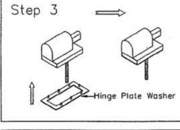
Attach the hinge rubberized plate washer to the bottom of the hinge mechanism.
