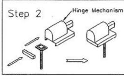
Slide the hinge plate into the underside of hinge mechanism. Insert the cover plate into the small nick.
