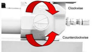
Turn valve clockwise on the pump until it is HAND TIGHT. DO NOT USE A WRENCH. Make strokes necessary to snap pipe. Turn knob counterclockwise to release valve after cut to retract piston.
