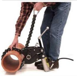
Using hand ring, pull chain over pipe and under tie bolt, then up between jaws as tightly as possible.
