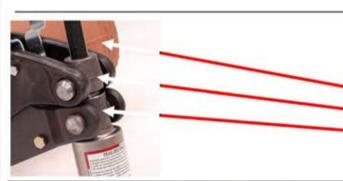
Turn adjusting screw until outer collar is at it's lowest limit of travel. Do this for EACH cut.
