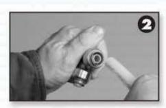
Step 2. SharkBite® push-fittings come with integral tube support liners. Ensure that the support liner is in place. The liner reinforces the wall of the PEX tubing to help prevent collapse of the tubing wall.
