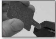
Gauge must stop at the NO-GO line in order to make proper connections
