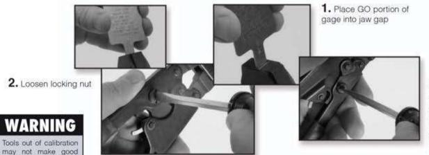
3. Adjust clamp tool jaws by rotating the eccentric stud counter-clockwise until jaws contact gauge. Re-tighten the locking nut.
