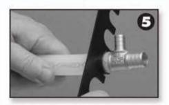
Step 5. Verify that the connection is secure by using the go/no-go gauge. The gauge slot that corresponds to the crimp ring size should easily slide onto the compressed crimp ring.
