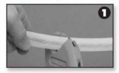
Step 1. Use plastic tubing cutters to cut the tubing to length, making sure that you have a good square cut. A rough or uneven cut will result in a weakened joint.
