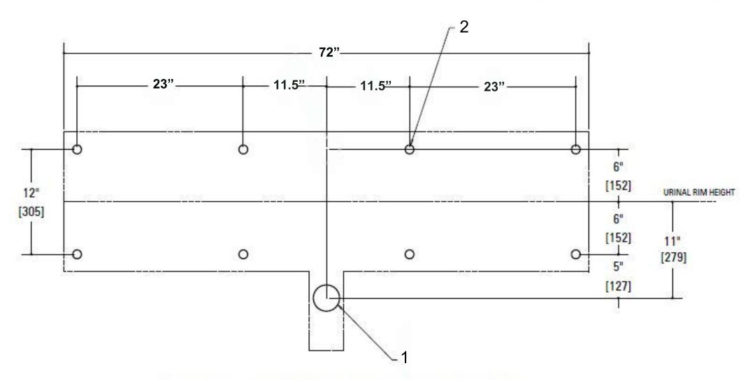
HOLES FOR CORE DRILLING OR STEEL PLATE WALLS
