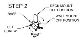
NOTE DEPTH OF SET SCREW PRIOR TO LOOSENING. LOOSEN SET SCREW AND ROTATE EYEWASH ARM 90°CLOCKWISE (AS SHOWN) WHILE MAKING SURE TO NOT ROTATE THE SPOOL, RE-TIGHTEN SET SCREW IN NEW POSITION. ENSURE SET SCREW IS PROPERLY SEATED IN INDENT. ENSURE SET SCREW IS TIGHT AND AT IT'S ORIGINAL DEPTH. ENSURE CORRECT ARM ORIENTATION BEFORE MOUNTING TO WALL. REFERENCE DRAWINGS AT RIGHT.
