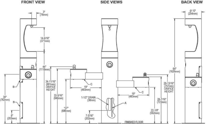
A = 3/8" O.D. Unplated copper tube connect. Shut off valve by others.
