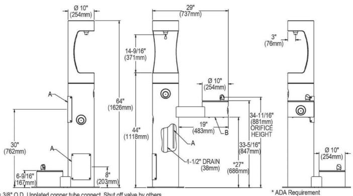
A = 3/8" O.D. Unplated copper tube connect. Shut off valve by others.
