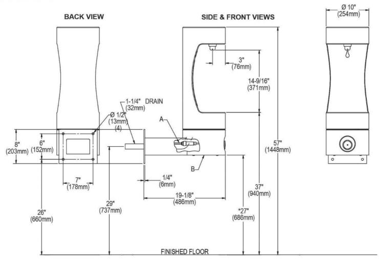
A = 3/8" O.D. Unplated copper tube connect. Shut off valve by others. B = Access panel(8" x 10")
