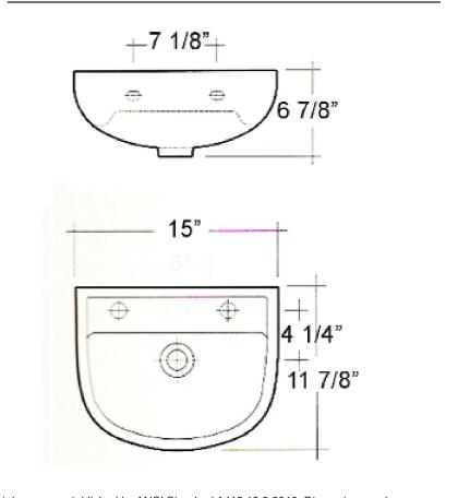
Dimensions of fixture are nominal and may vary within the range of tolerances established by ANSI Standard A112.19.2.2013 Dimensions and specifications subject to change without notice.
