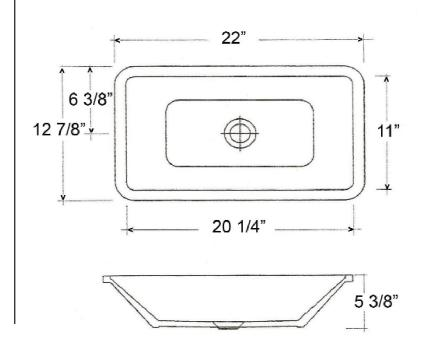
Dimensions of fixture are nominal and may vary within the range of tolerances established by ASME Standard A112.19.2.2013 Dimensions and specifications subject to change without notice.
