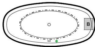
Factory installed blower may only be placed in this location.
