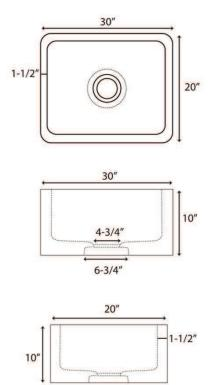
Dimensions of fixture are nominal and may vary within the range of tolerances established by ANSI Standard A112.19.2. Dimensions and specifications subject to change without notice.
